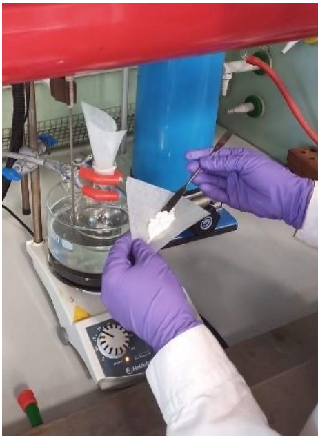
Figure 11: cellulose-based white pigment to replace the controversial, but most widely used white pigment, titanium dioxide (TiO 2 ) (Cellulose White Pigments From Impossible Materials | | AWRD (Ja), n.d.)
